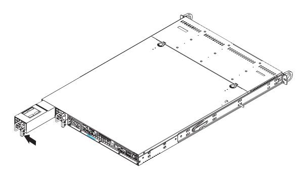
Figure 6-6. Removing/Replacing the Power Supply
